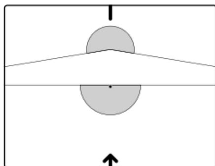
The Caproni Ca.3 has a higher rear machine gun platform with no blind spot. The drawback to having such a platform is that the rear gunner is very exposed to enemy fire.
